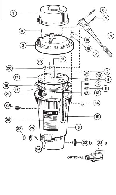
Screw the fitting into the thread hand tight; then, using a wrench, tighten one more full turn. Additional tightening is unnecessary and could result in broken or damaged fittings.
